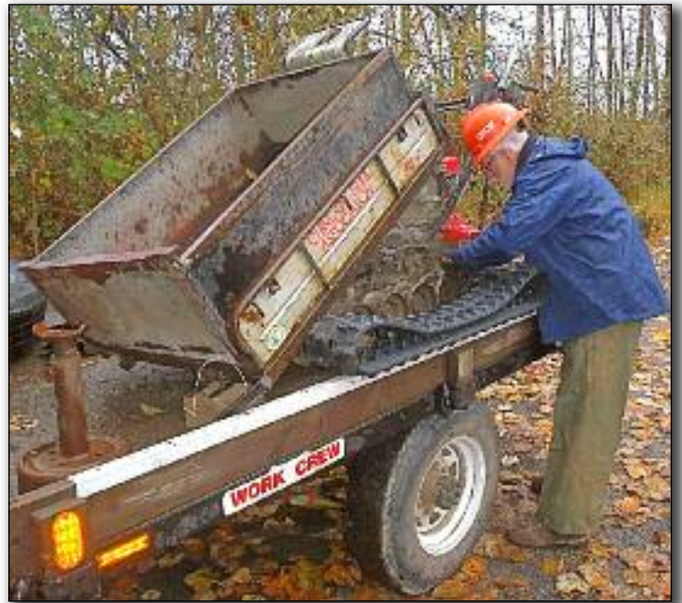
Dick Blackburn installs new track on a CTA tote. (Photo by Ted Klump)
